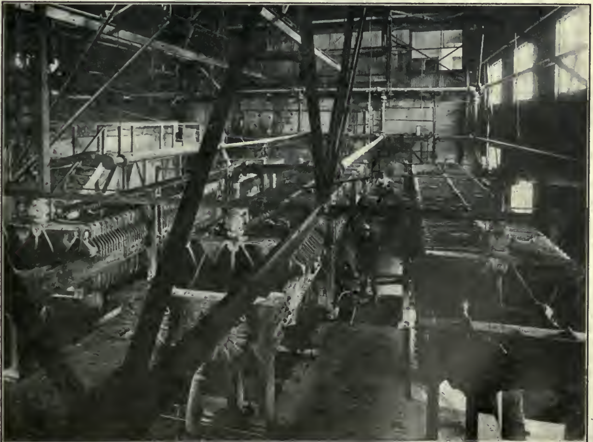
MERRILL PRESSES AFTER ENLARGING TO 86 FRAMES, PITTSBURG SILVER PEAK.
